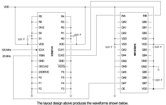
Note: Series terminating resistors are not shown.
